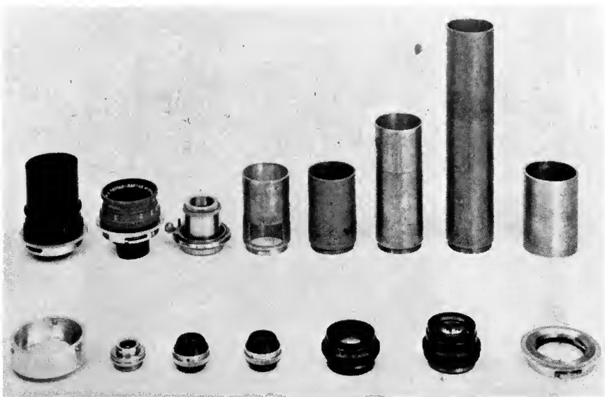
Fig. 1. Lenses, adapters, and extension tubes used with the Fastax camera.
